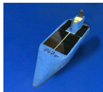
CATS-SATag with optional solar re-charge
